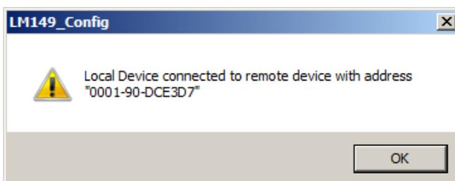
⇒ Disconnect the adapter from the computer and connect it to the target device (e.g. a balance). Remember to adjust the setting of the DCE-DTE switch as needed.
